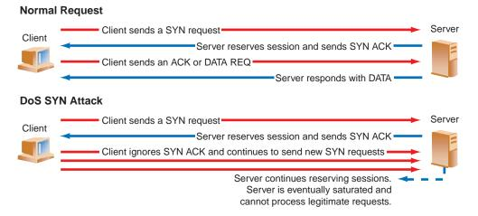
Figure 6-9 DoS SYN Attacks without Delayed Binding
